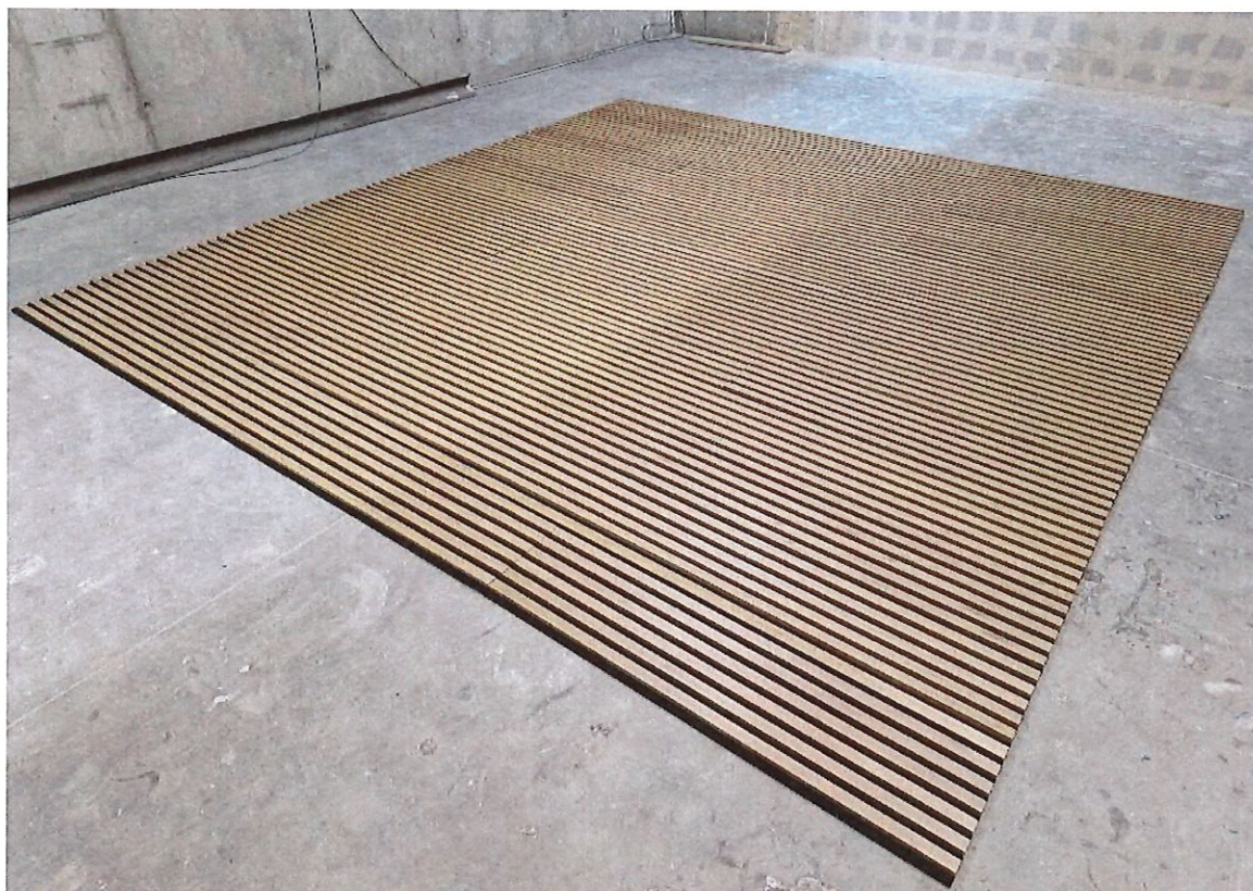
Figure. 2. Photo showing decorative acoustic panels. Test specimen No: GLA-1664/ 24 mounted on the test bench. Photo by Gryfitlab
