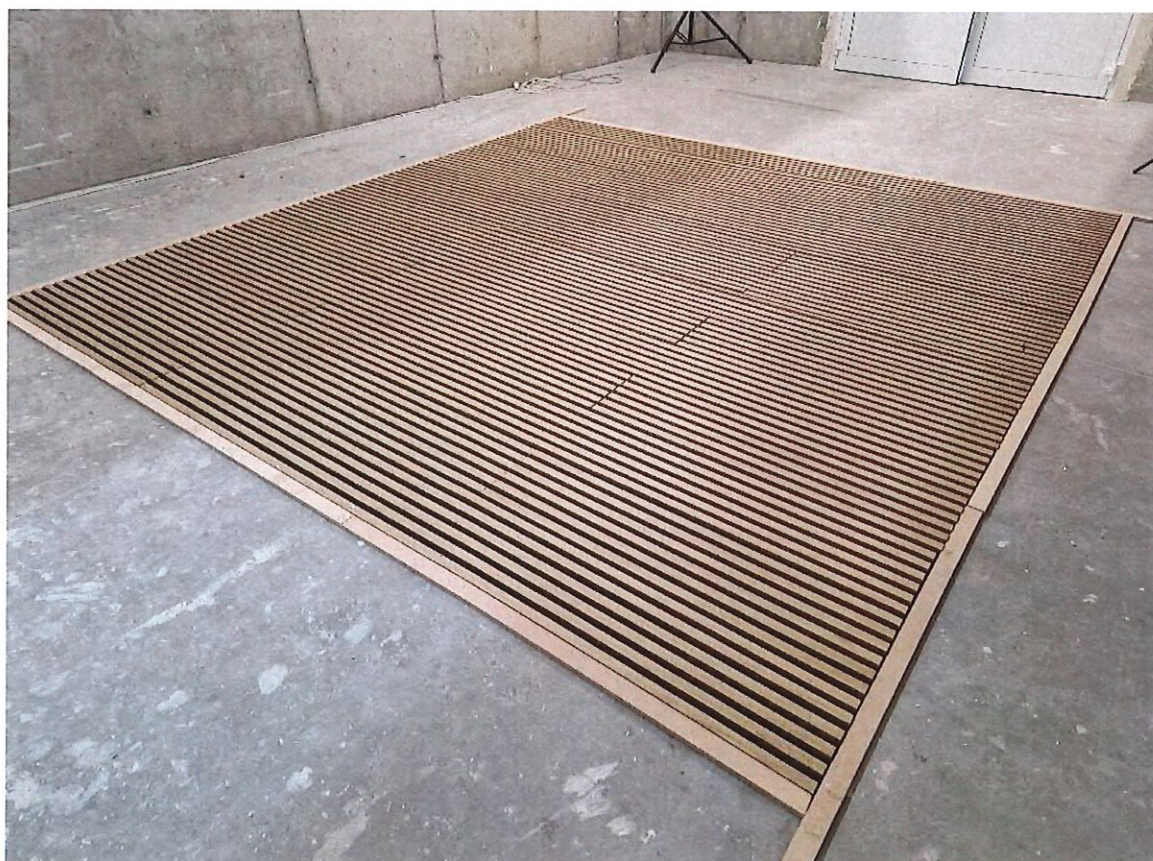
Figure. 3. Photo showing decorative acoustic panels. Test specimen No: GLA-1664/ 24 mounted on the test bench. Photo by Gryfitlab
